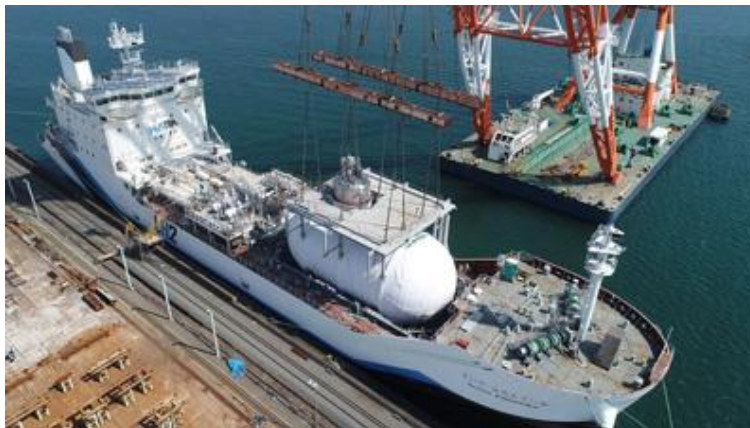
Figure 4: Liquid hydrogen transportation vessel (Source: Kawasaki Heavy Industries)
